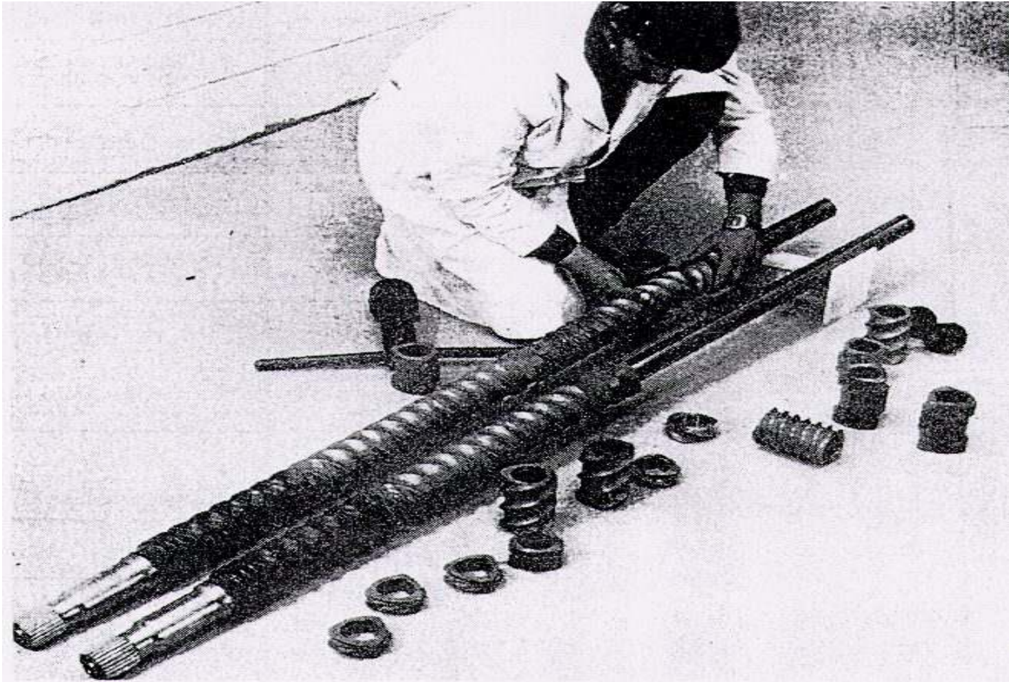
Figure 2.4 A Werner & Pfleider screw assembly offers specialized processing combinations.
